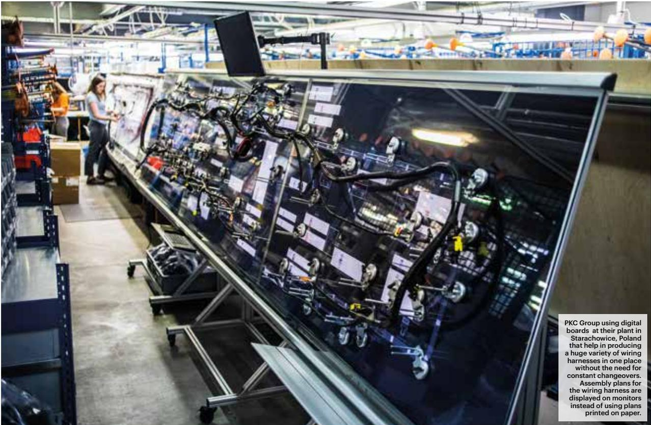
PKC Group using digital boards at their plant in Starachowice, Poland that help in producing a huge variety of wiring harnesses in one place without the need for constant changeovers. Assembly plans for the wiring harness are displayed on monitors instead of using plans printed on paper.
